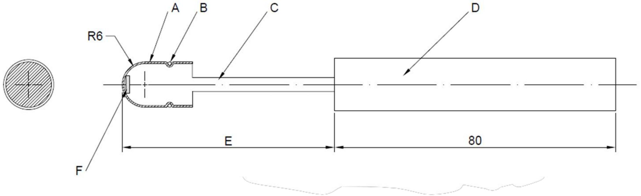
**TESTING FOR UNINTENDED ACCESS TO A SHARP, ONCE THE SHARPS PROTECTION MECHANISM IS IN 'SAFE MODE' (BY USING AN ARTIFICIAL FINGER)**
